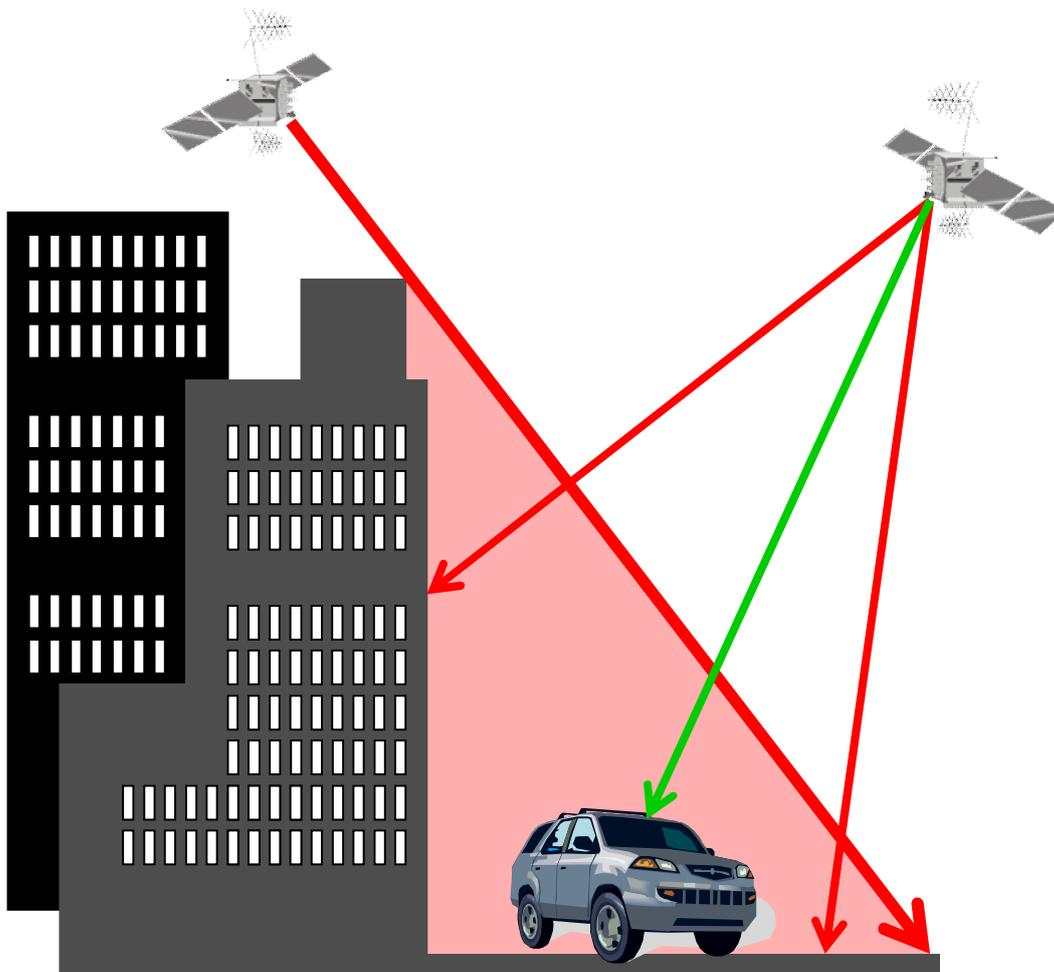
Figure 3 – Severe reduction of satellite reception in Urban Canyons
