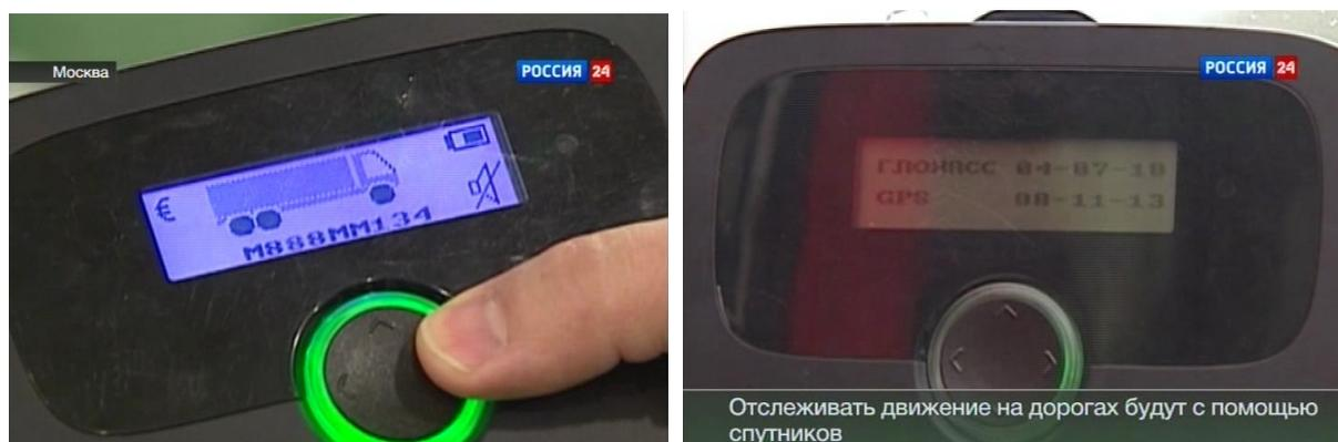
Figure 3 – Demonstration of the GPS / GLONASS OBU Functionality in Moscow, in which also the simultaneous reception of GPS and GLONASS signals can be viewed in real-time (right) <sup>2</sup>
