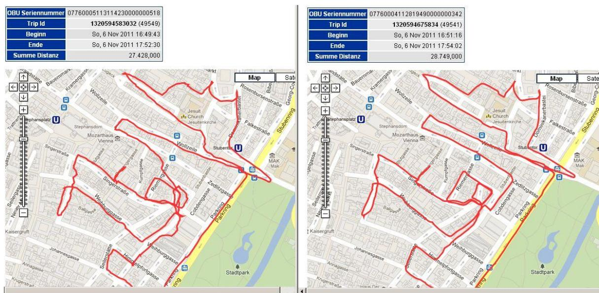
Figure 4 - A trip through the center of Vienna's Historical Center with a GPS-only OBU (left) and a combined GPS/GLONASS OBU (right)
