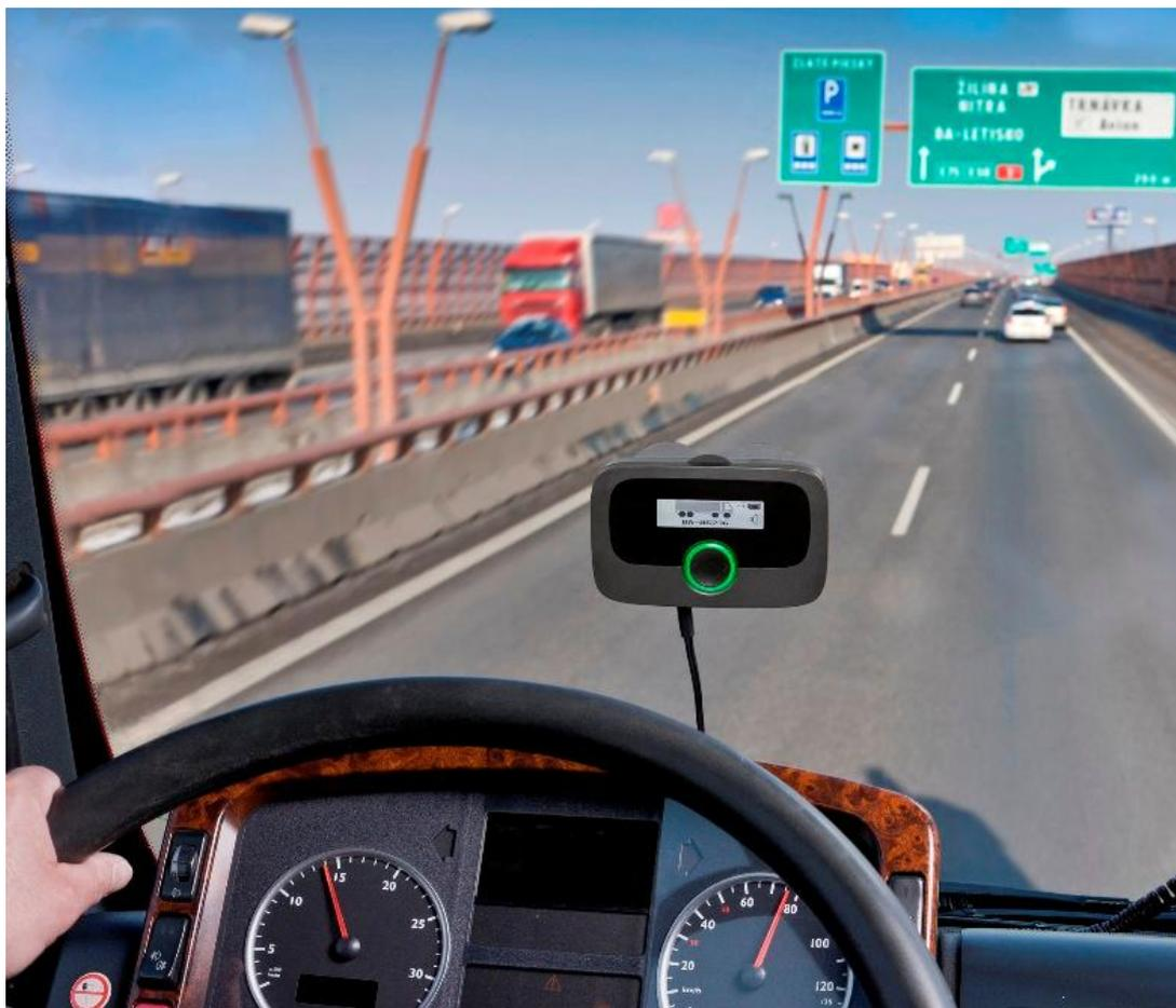
Figure 1 – Windshield-installed GNSS *Sensus Unit* used in Slovakia (and soon also in France)
