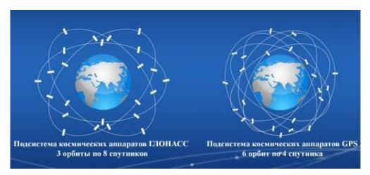
Figure 5 - The orbits of GLONASS Satellites (left) and of GPS Satellites (right)
