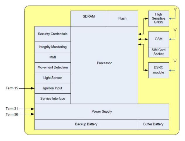
Figure 3: Block Diagram of the OBU Hardware Components
