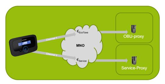
**Figure 5: Potential Service Proxy Architecture**
