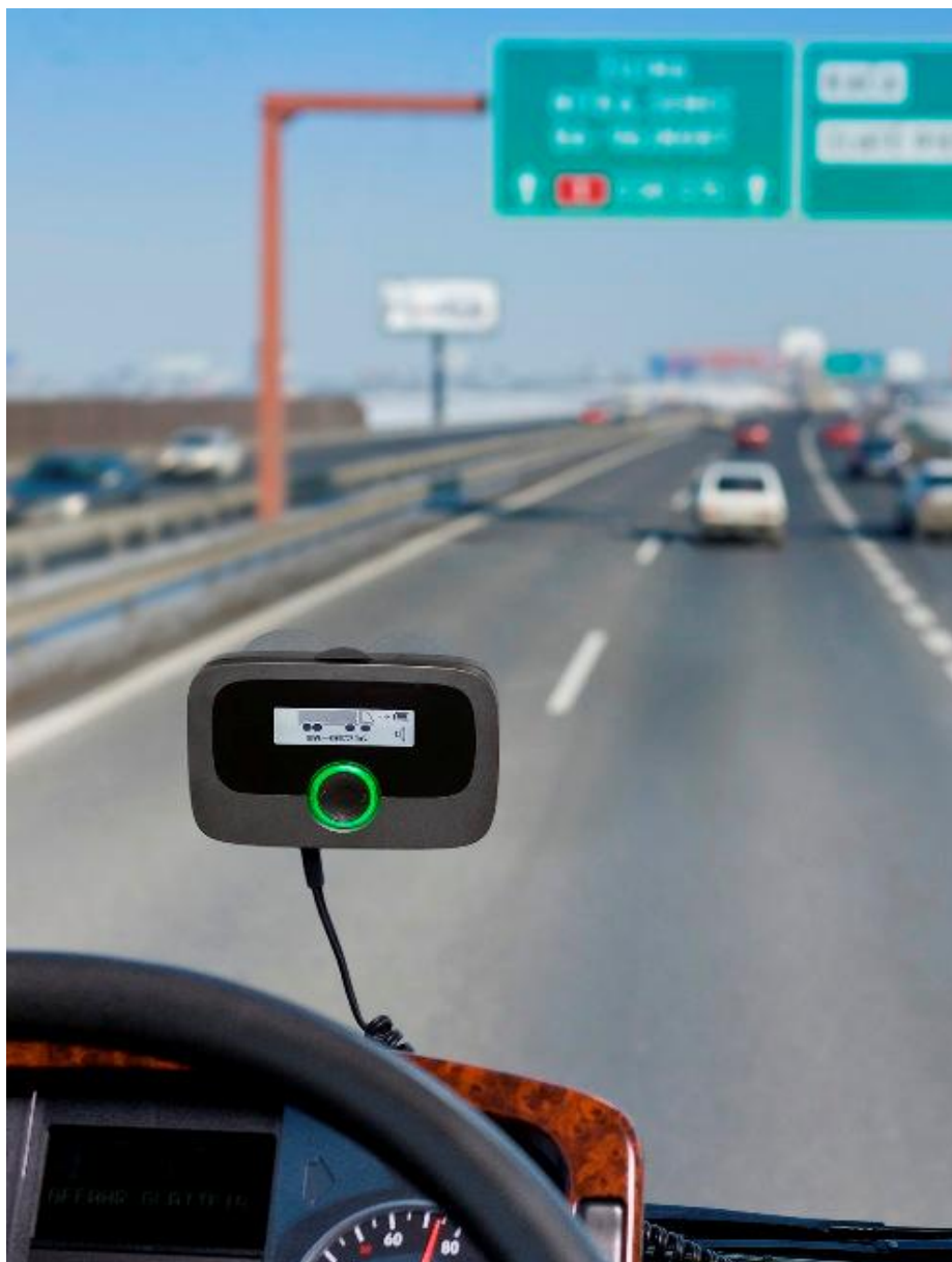
Figure 3 – The second generation “plug and play” GNSS OBU used in Slovakia
