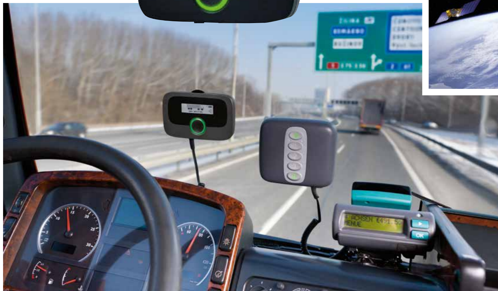
(Left) Three types of GNSS-based OBUs on a vehicle's windshield (Above) The Galileo satellite system
