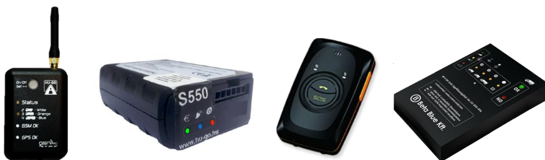
Figure 2 - Some of the Fleet Management Tracking Devices Used in the Hungarian Toll System
